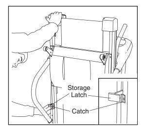
2. Hold the treadmill firmly with both hands, and lower the treadmill to the floor. Do not drop the treadmill frame to the floor. To decrease the possibility of injury, bend your legs and keep your back straight.
